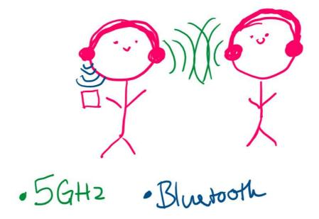
The physical design of this solution mimics a standard headset. Ideally, people would not notice the difference between the proposed solution and an off the shelf version, except for the added functionality. Each of the headsets should be exactly the same, so they each can be used normally on their own, but can act as a mesh network of headsets if multiple are used.
