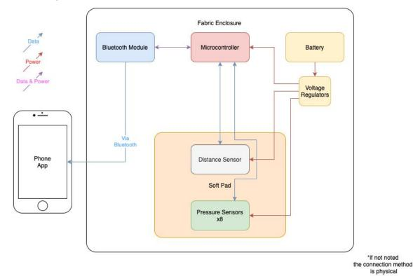
After the battery voltage is regulated the microcontroller reads the data from the eight pressure sensors and one distance sensor and packages the data to be sent off via the bluetooth module. The module then sends the data to the phone application. The phone application takes the raw data and converts it into a display for the user to actively monitor their seating position.
