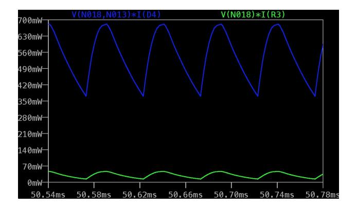
This chart shows the power consumption for a single LED vs the current limiting resistor, which is what led to the double LED design. Originally, we were using a single LED vs the resistor and there were large losses through the resistor. By doubling up, we not only required less components, but our efficiency increased as the resistor was able to current limit two LEDs. The double LED design also pushed down the voltage drop on the resistor thus further dropping its power consumption.
