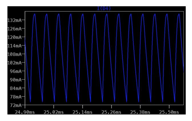
This is the estimated "safe" levels of current that we would be able to push into the LEDs. This current ripple stays below the absolute rating of 150 mA and gives us an average of around 100 mA. We may be able to push this higher as needed, but we currently do not think the trade off will be worth it.
