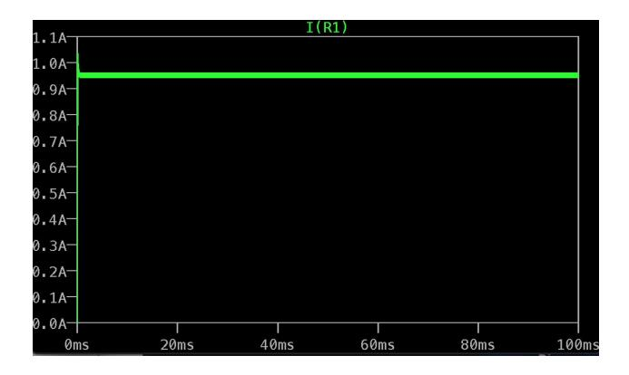
This is the simulation of the current into the motors. This falls roughly in the ballpark of what we would expect from our motors. This is less important on its own due to the estimated nature of our motor parameters, but is useful for determining load on the battery pack.
