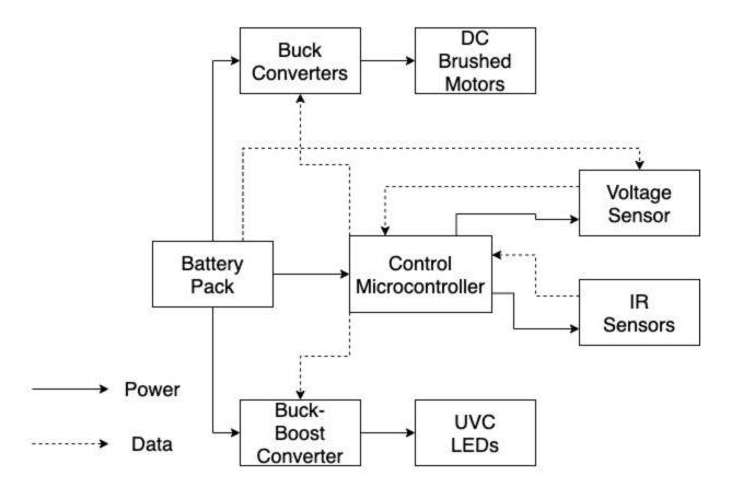
**Battery Pack** - This will be a 3 cell Lithium ion pack that will power the device. Since this is a 3 cell pack, it will have a voltage range between 9-12.6v. We are looking at powering 10 LED modules, 2 DC motors, and an Arduino for about an hour. This gives us an estimated capacity of 13 Ah for a worst case scenario. Realistically, the motors will not be running constantly at full throttle, so a more realistic range would be 10-12 Ah.
