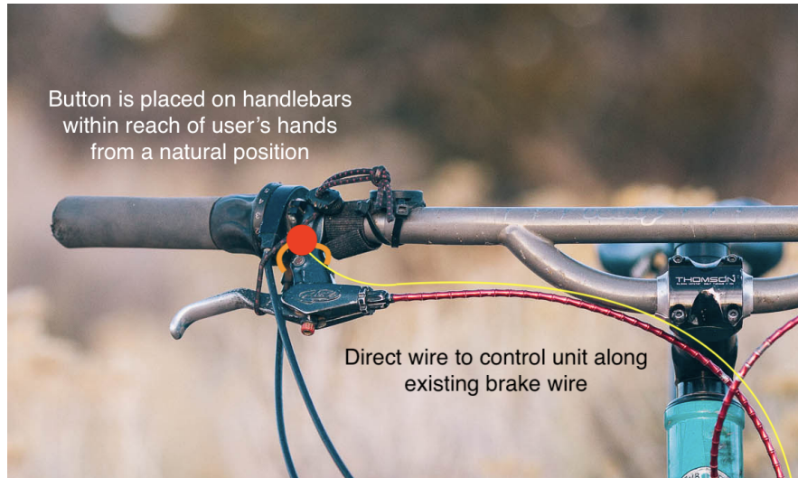
Figure 2: Diagram showing how a turn signal button will be mounted on a bike's handlebars so that a user can activate the turn signals.
