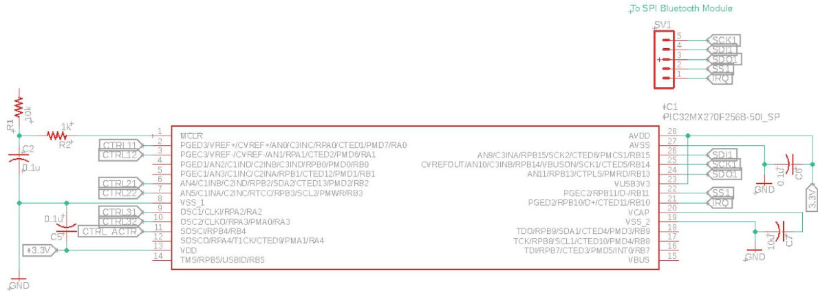
Diagram for Control Module Circuit (MCU)
