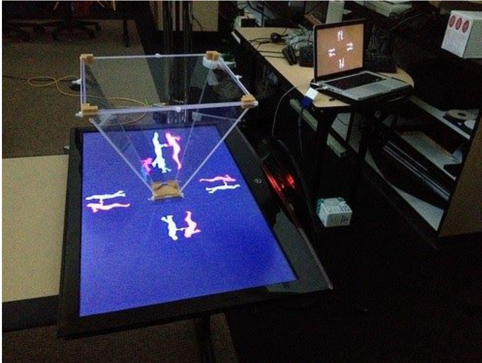
Figure 4: A functional test of a holographic display reflecting the screen images
