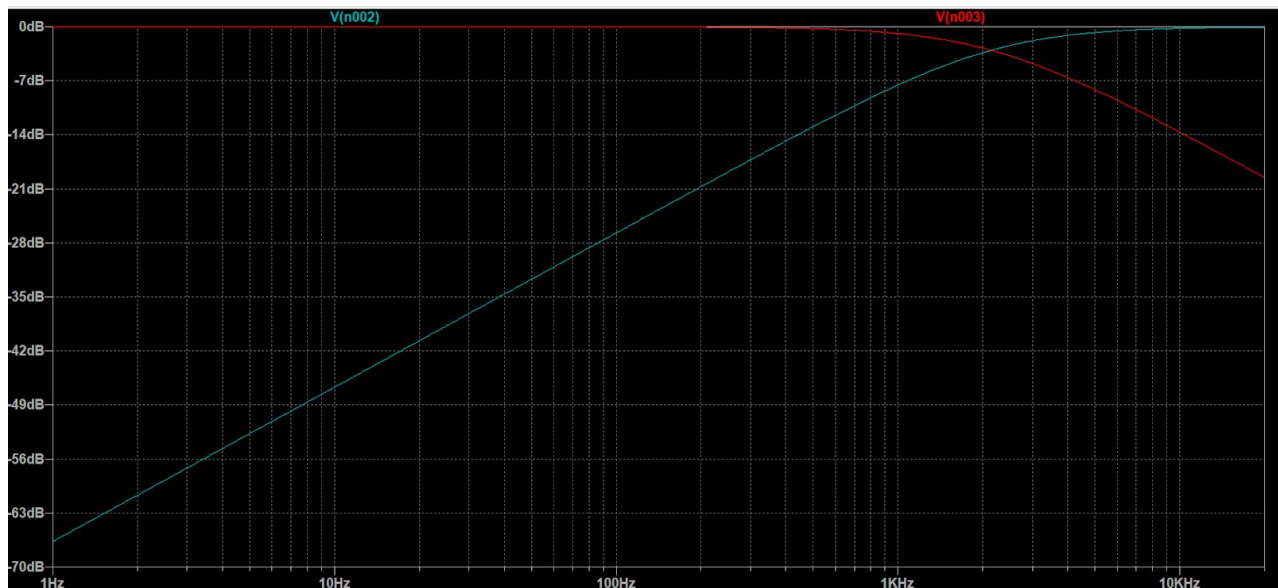
Figure 5: LTSpice Simulation Results of Crossover Schematic with crossover at 2.15kHz
