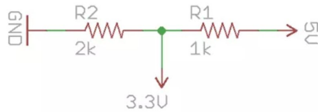
Figure 7: Circuit diagram of the voltage divider
