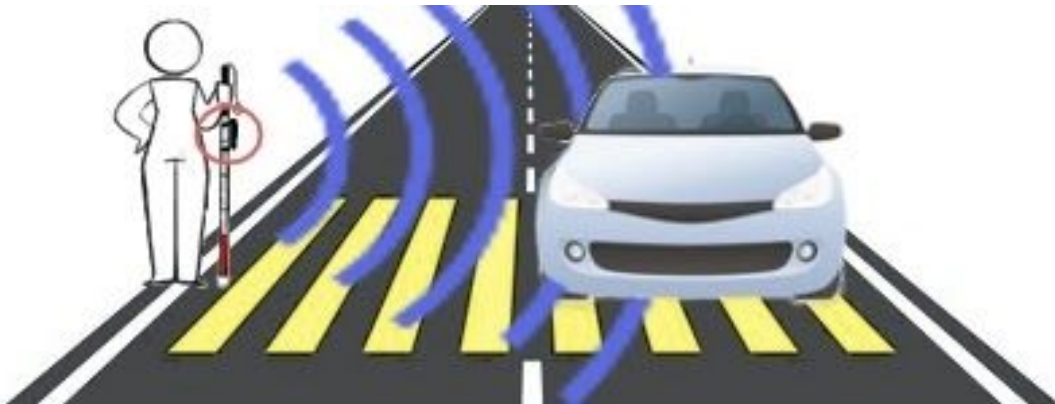
Fig 1: Visual Aid: When the user approaches a crosswalk, they can activate the vehicle detection cane attachment (circled in red) which will use a doppler radar to detect oncoming traffic (represented with blue lines). If a vehicle is detected, then the device will notify the user through vibration feedback.
