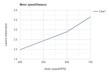
The graph above is the motor speed/Launching distance graph at a fix 10 degree launching angle
