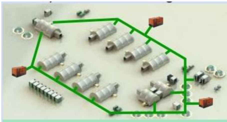
Figure 6: Physical Layout of a Tactical Microgrid Application [1]
