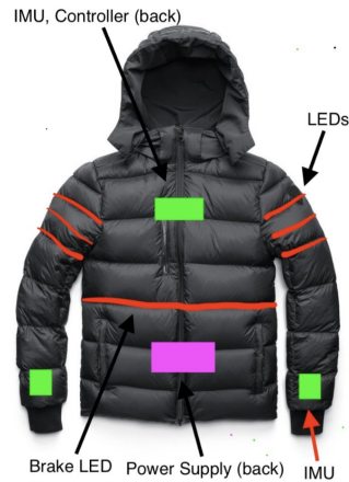
Figure 3: Diagram of how our design will be physically laid out on a jacket.
