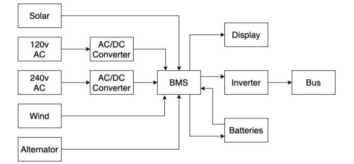
The high-level, power flow block diagram. Most of these components will be bought off-the-shelf. The primary exception will be the central BMS system. We will be constructing that as our PCB.
