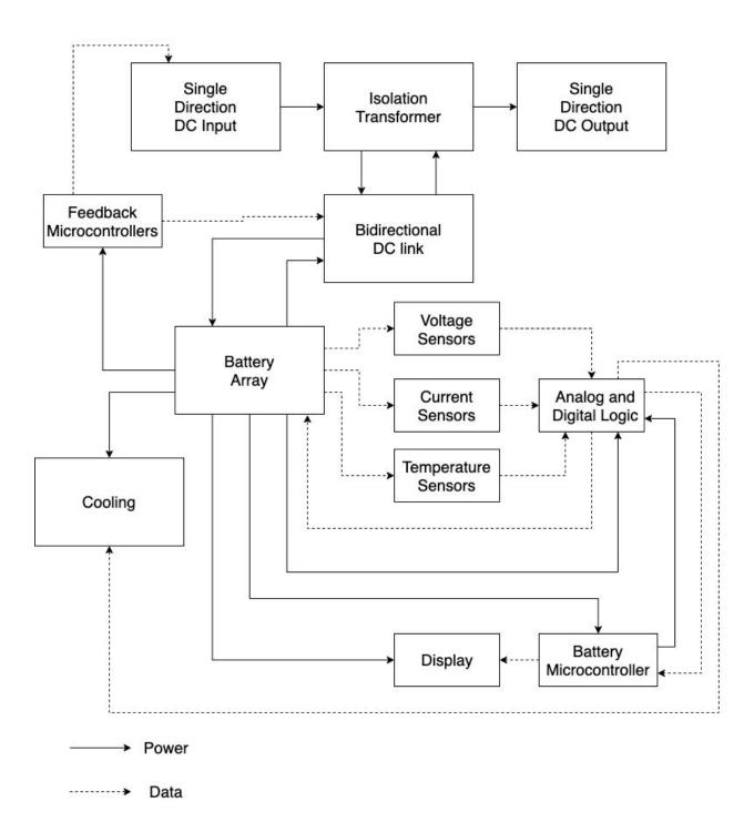
The BMS block diagram. We will be making most of these components on multiple PCBs. Some of these components, such as the cooling and microcontrollers, will be bought but then configured to fit our project.
