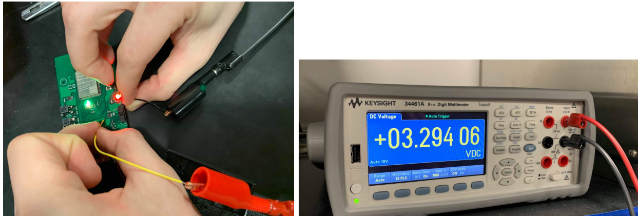
Figure 9 Measuring the voltage output of the AP2112K 3.3 V voltage regulator from the IMU USIC controller (on the left) with a lab bench digital multimeter (on the right).
