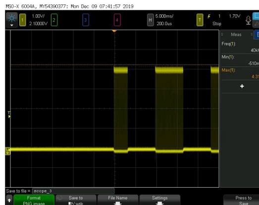
Figure 13. Modulated Signal
