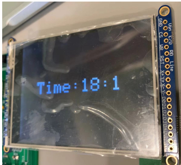
Figure 12. LCD Displays Correct Time with RTC Data
