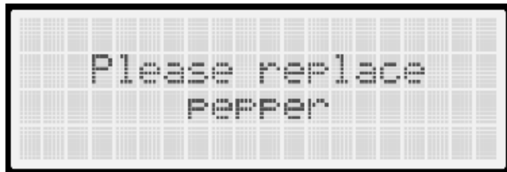
Figure 13: Replace seasoning screen. The seasoning name will change to whichever seasoning must be replaced. If both need to be replaced, will list both on the same line separated by a comma.
