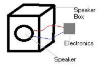
To ensure we do not have to fine-tune the physical speaker design, we will use a pre-existing speaker and speaker box setup with pre-tuned acoustics which will connect to our PCB (Printed Circuit Board). Our PCB will be connected to wall power to optimize current for powering the speaker and long testing cycles when finetuning EQs. Since the Bluetooth communication to the control subsystem is a preexisting digital device, i.e. phone or computer, we have not included it in our physical design.
