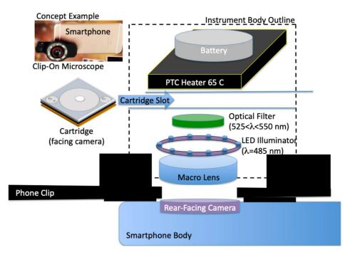
The instrument is comprised of a macro lens, a ring-shape LED illuminator, an emission filter, a PTC (positive temperature coefficient) heater, a rechargeable battery, and a clip-on container. The system fits over the rear-facing camera of a smartphone and has a slot to accept the test cartridge after reagents are added. Physical design picture credits to the PFI Proposal provided by Prof. Cunningham.
