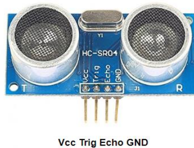
Figure 2.2 Ultrasonic Sensor and its pin out
