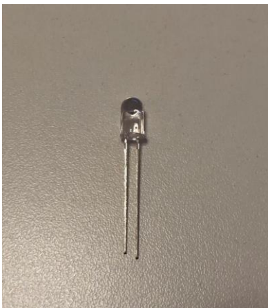
Figure 2.5 970 nm IR transmitter
