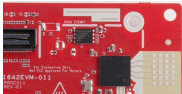
Figure 3. Slot Antenna Array Design with Coupon Structure for a Probe by TI [8].
