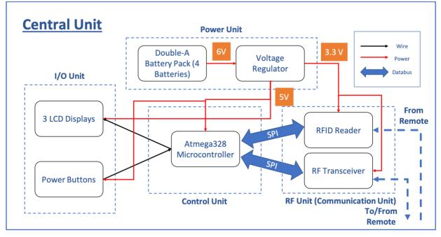
Figure 1: Block Diagram of Central Unit
