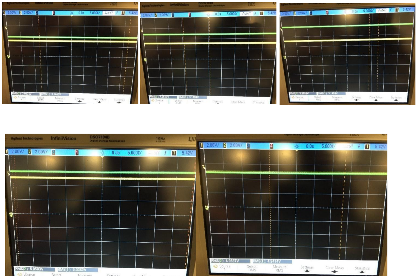
Figure 16 LDO (3.3V) Output Waveform (a) 5V Input (b) 6V Input
