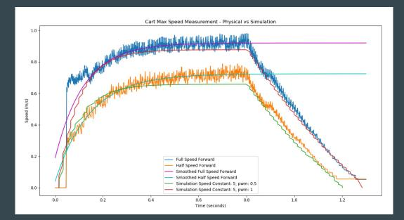
• Best fit line to exponential function  $y = A - Be^{-Cx}$  for rising velocity of motor, fit using scipy optimize function
