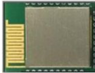
Figure 4: CYBLE-214015-01 EZ-BLE chip
