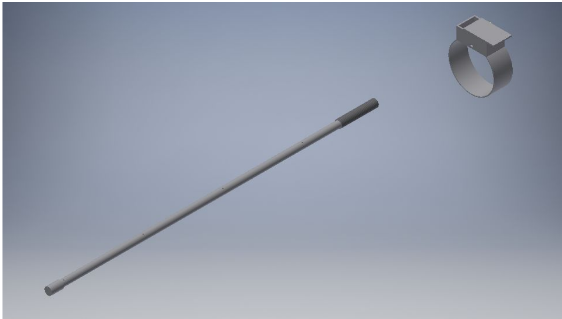
Figure 2. 3D rendering of white cane assembly with wearable bracelet.
