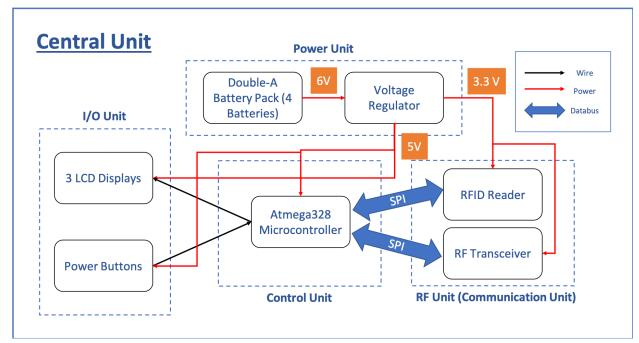
Figure 1: Block Diagram of Central Unit
