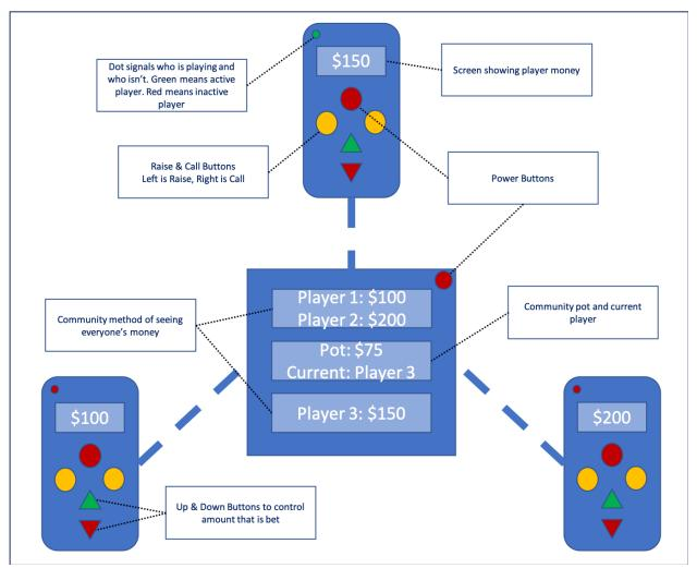
Figure 3: Physical Layout of Full Apparatus
