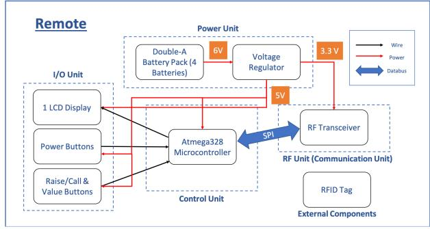
Figure 2: Block Diagram of Remote Unit
