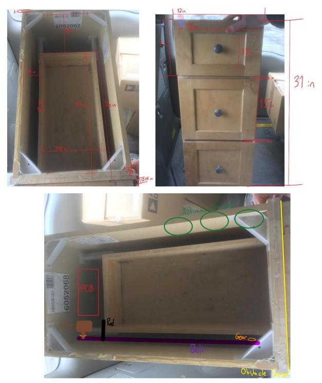
We have acquired the above dresser from Habitat for Humanity ReStore. We chose it because it has ample space behind and around the drawers for motor, belt, power, and PCB installation. The belt (purple) will extend from the gear (orange) around the motor shaft to the gear near the front of the dresser for maximum extension. The motor (brown) will be mounted on the
