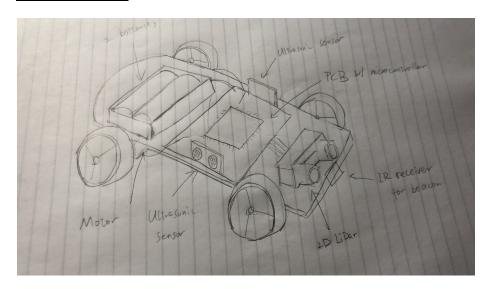
Physical structure description: Our chassis will contain two batteries as DC power supply, two motors, two ultrasonic sensors, a 2D LiDar and an IR receive for beacon, and all
