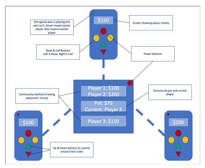
Our physical design consists of essentially a main display device and the remote(s) for each player. On the main display we plan to display:
