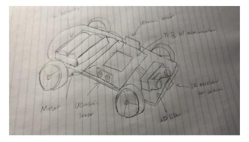
Our chassis will contain two batteries as DC power supply, two motors, two ultrasonic
