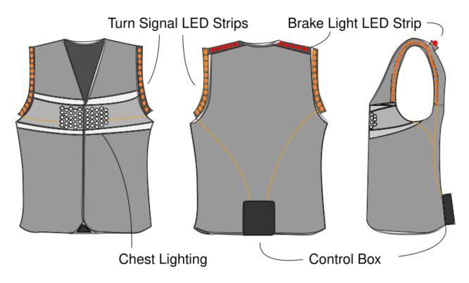
The entire device is integrated into a one size fits all vest. Over the shoulders and along the upper back are RGB LED strips with each light individually controllable.
