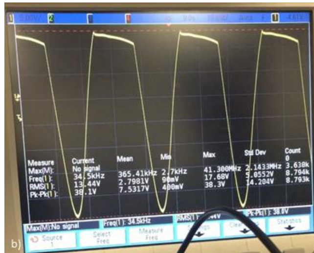
Figure 4: Measured voltage across primary coil. The linear region occurs because the mosfet is not switching at the resonance frequency of the primary coil and C 2 capacitor.
