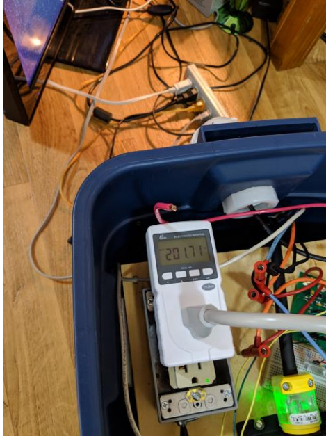
Figure 15. 200 W Battery Capacity Verification Setup
