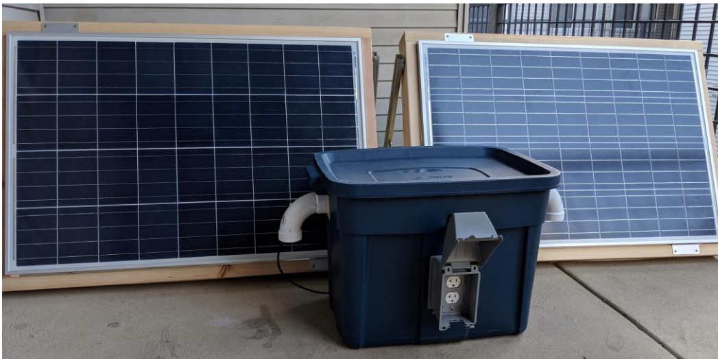
Figure 4. Off-Grid PV Generator Overall Physical Design
