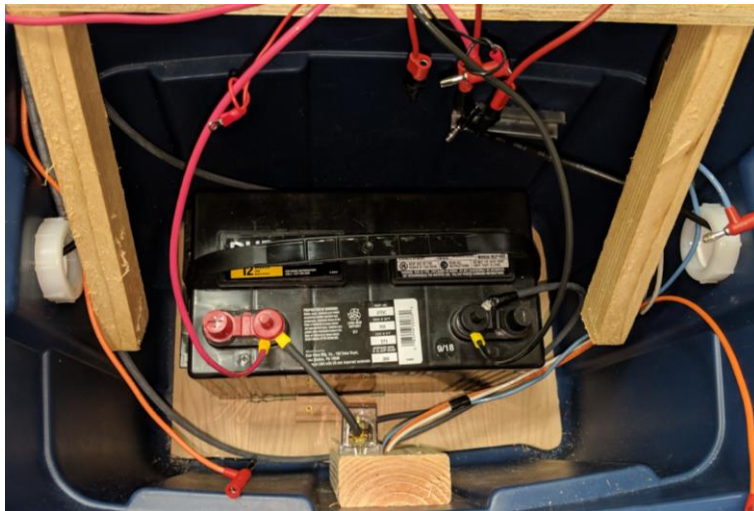
Figure 16. Wooden Battery Support
