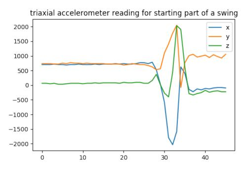
The horizontal axis is the number of samplers and since sample rate is 10Hz, one can
