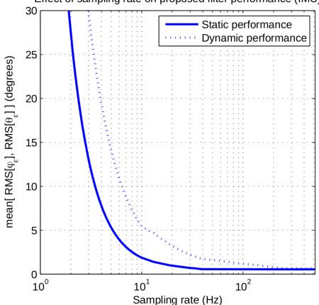
Effect of sampling rate on proposed filter performance (IMU)
