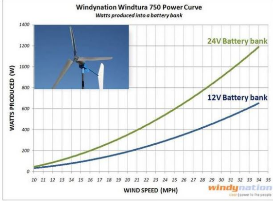
Figure 5: Power vs Wind Speed curve for the Windynation 750 PMA
