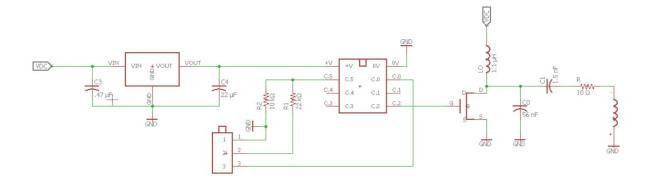
The charging circuit is composed of two major parts the primary and secondary sides. The primary side consists of a 12V 1A AC-DC wall adapter, a 5v voltage regulator, a square wave frequency generator (PICAXE), and a Class E Inverter to produce a sinusoidal current. The secondary side has a receiver coil that has an induced current and a full bridge rectifier to convert the AC wave into a DC voltage. It also contains another voltage regulator and a battery charging IC.
