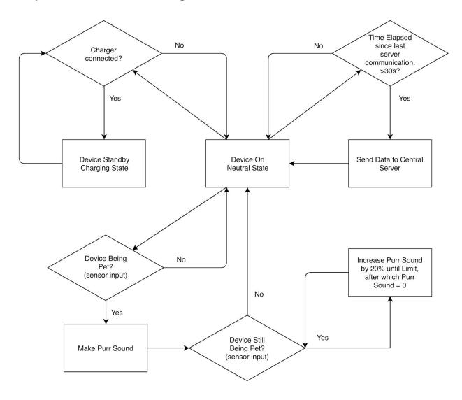
The control block diagrams above satisfies the high level requirements. The charging control flow will verify if the device is charging successfully or not when it goes to Standby state. Processing and routing of sensors is verified by touch input and corresponding purr sounds. Sending of diagnostic data is indicated by the 30 second transmit loop.
