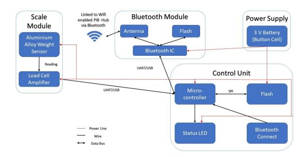
Figure 3. Block diagram for Pill Scale
