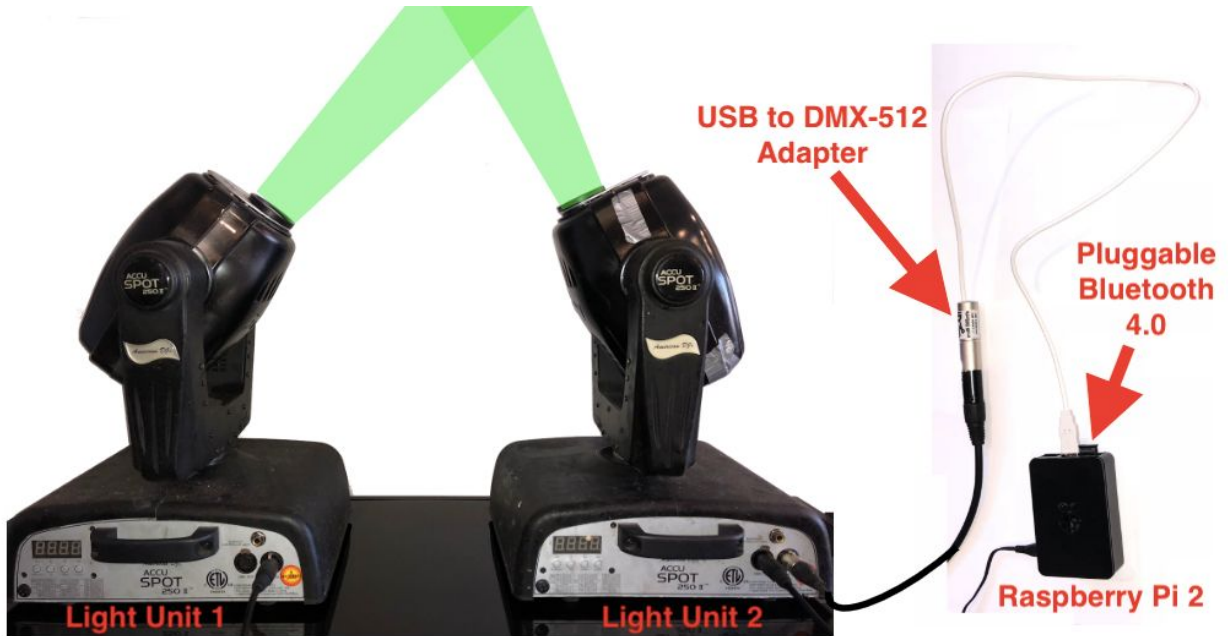
Figure 13: Picture of the Main Control Unit attached to the Light Units.
