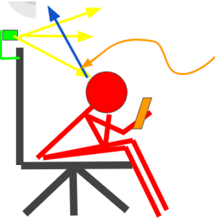
Figure 10 Ultrasonic measuring at an angle. The wave is reflected away from the sensor, which results in inconsistent/garbage readings.
