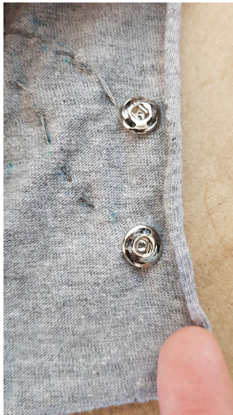
Figure 15. Wearable sleeve physical design (sewable conductive snaps).
