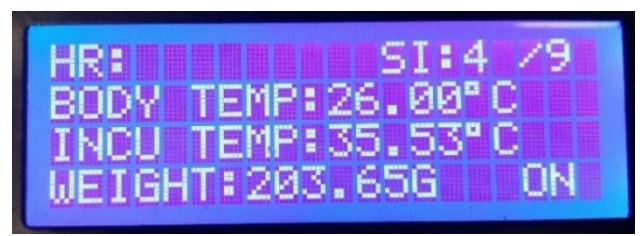
Figure 2.3.6d: Display Showing Temperature Below 36^{\circ}\text{C} . The display shows that when the temperature is below the threshold, the heating pads are turned on.
