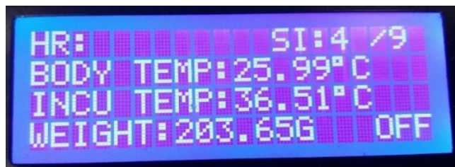
Figure 2.3.6c: Display Showing Temperature Above 36^{\circ}\text{C} . The display shows that when the temperature is above the threshold, the heating pads are turned off.
