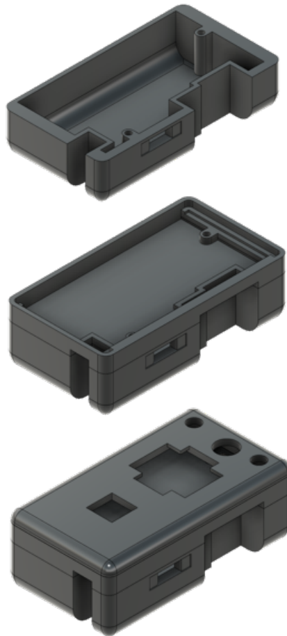
Figure 10: Main device enclosure design
