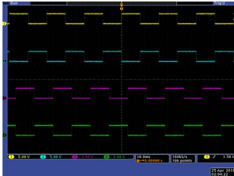
Figure 17: PWM Waveforms for Inverter
