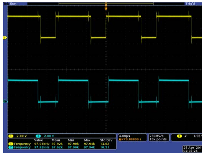
Figure 16: PWM Waveforms for Converter
