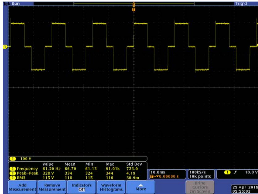
Figure 15: Inverter + Transformer Output Waveform with 3 rd Harmonic Eliminated
