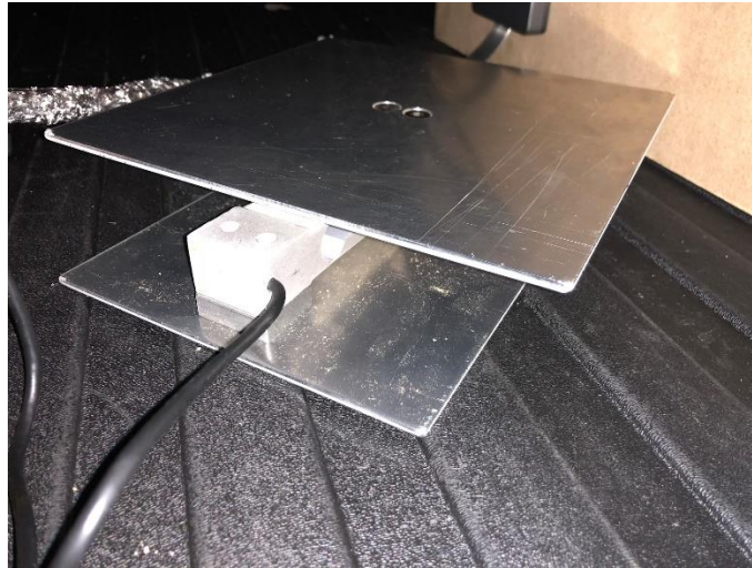
Figure 4 Picture of the load cell with platform built by the ECE Machine Shop.
