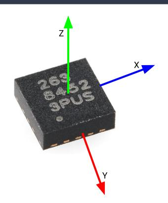
MMA8452 3-axis accelerometer:
