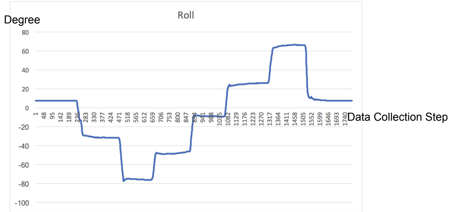
Fig 8. Roll against time-steps as measured from holding the breadboard at different angles
