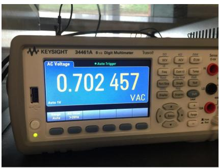
Test using 2V peak to peak sinusoidal waveform. efficiency = 99.3% at both channel
