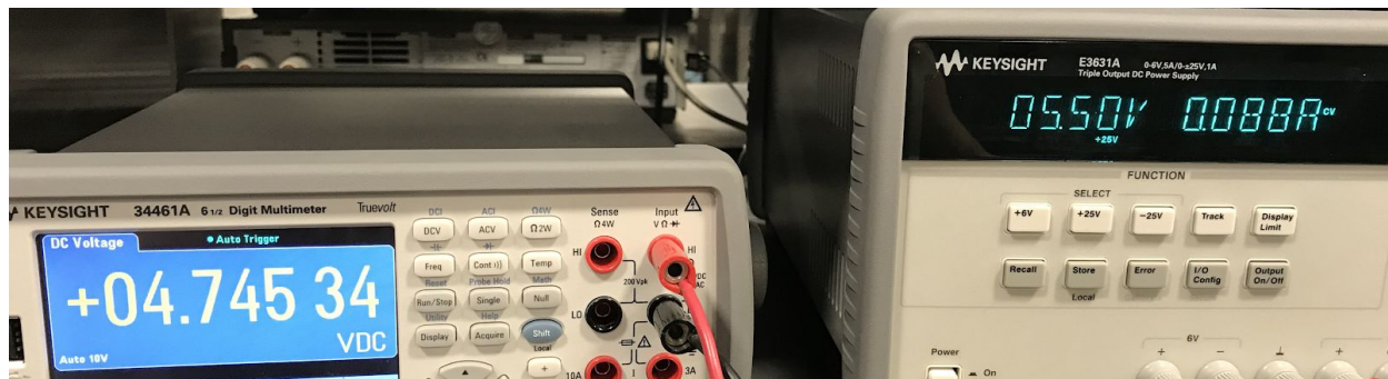
Figure 6: Output of the 5V voltage regulator given 5.50V input
