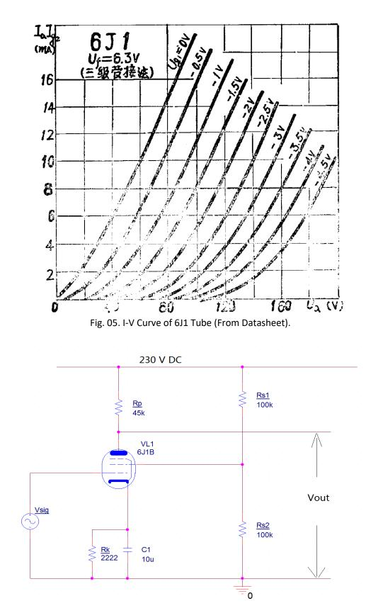
Fig. 06. Actual Circuit Diagram Consisting 6J1 Tube.
