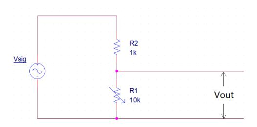
Fig. 03. Circuit Diagram Shows Volume Control Module
