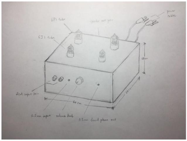
Fig. 02. Physical Diagram
