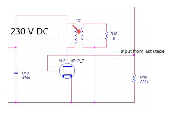
Fig. 09. Circuit Diagram Showing the Power Amp Stage
