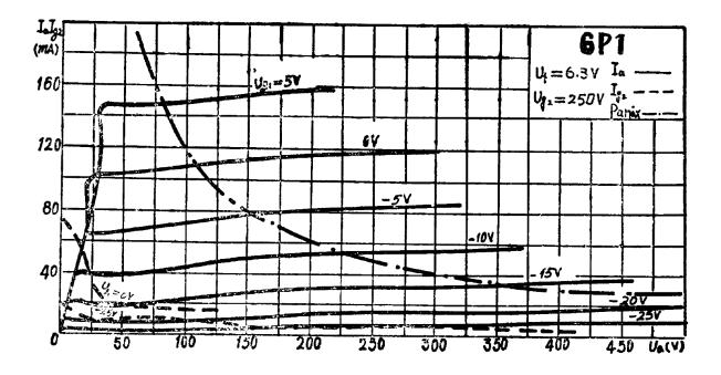
Fig. 08. I-V Curve from 6P1 Datasheet
